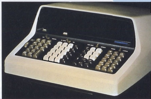
1968 —The HP 9100A (the world's first programmable scientific desktop calculator) was 10 times faster than most machines at solving science and engineering problems.
