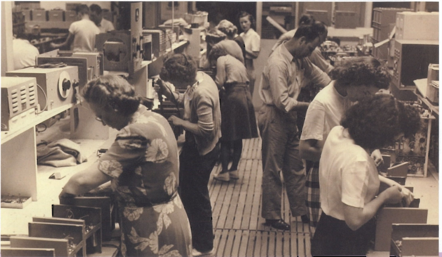
1946 —Ed Porter and Cecil Woods (rear center) view HP's "pass on" type of line assembly pioneered in the early years. It is HP's first manufacturing line at the Redwood Building, 395 Page Mill Road, Palo Alto, California, with audio oscillators and HP 300A wave analyzers.
