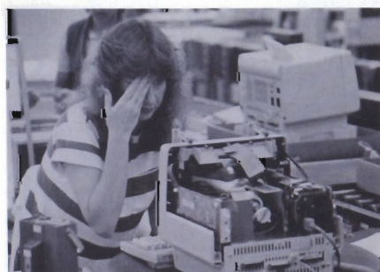
Ellen Price, a production worker at HP's Sunnyvale, California, facility, closes one eye to more effectively check the raster alignment of a touchscreen personal computer.
