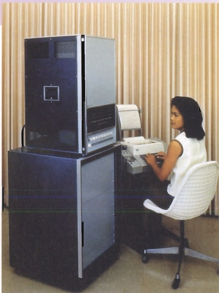
1966 —HP entered the computer market with the invention of the HP 2116A, designed as a controller for the company's test-and-measurement instruments.
